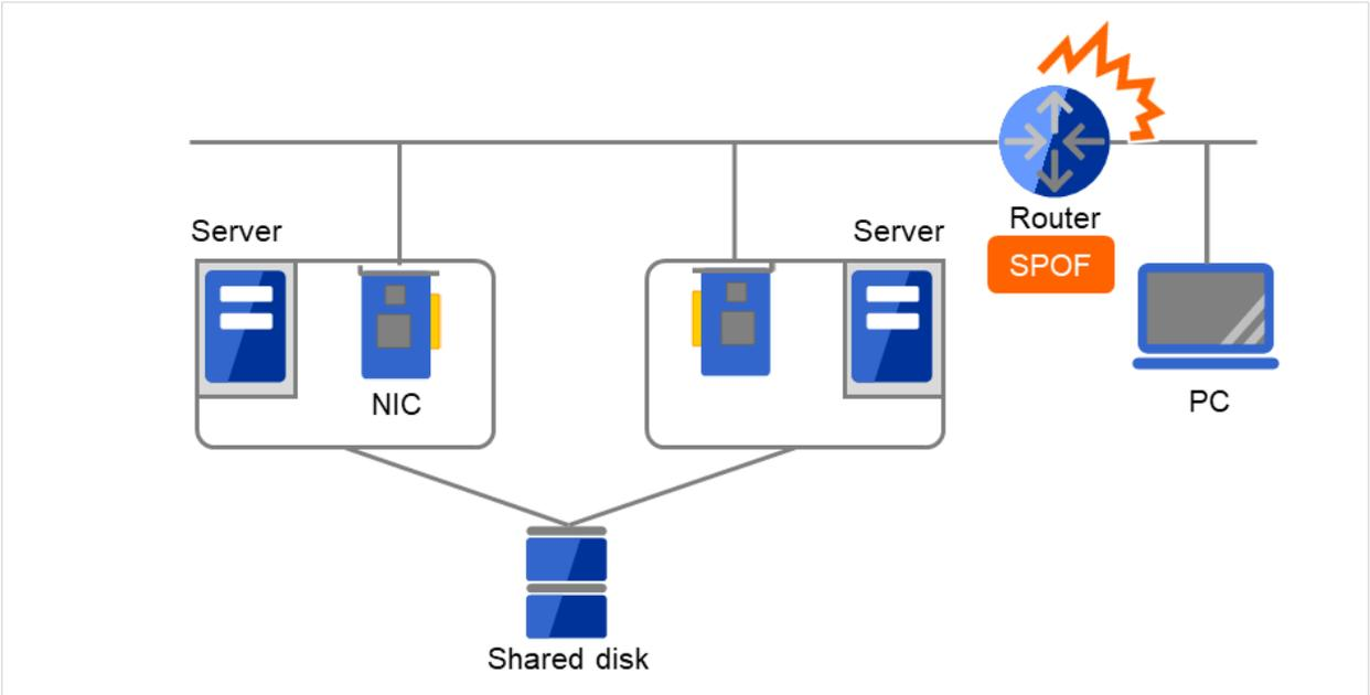
Fig. 2.22: Example of a failure with LAN (Router)
