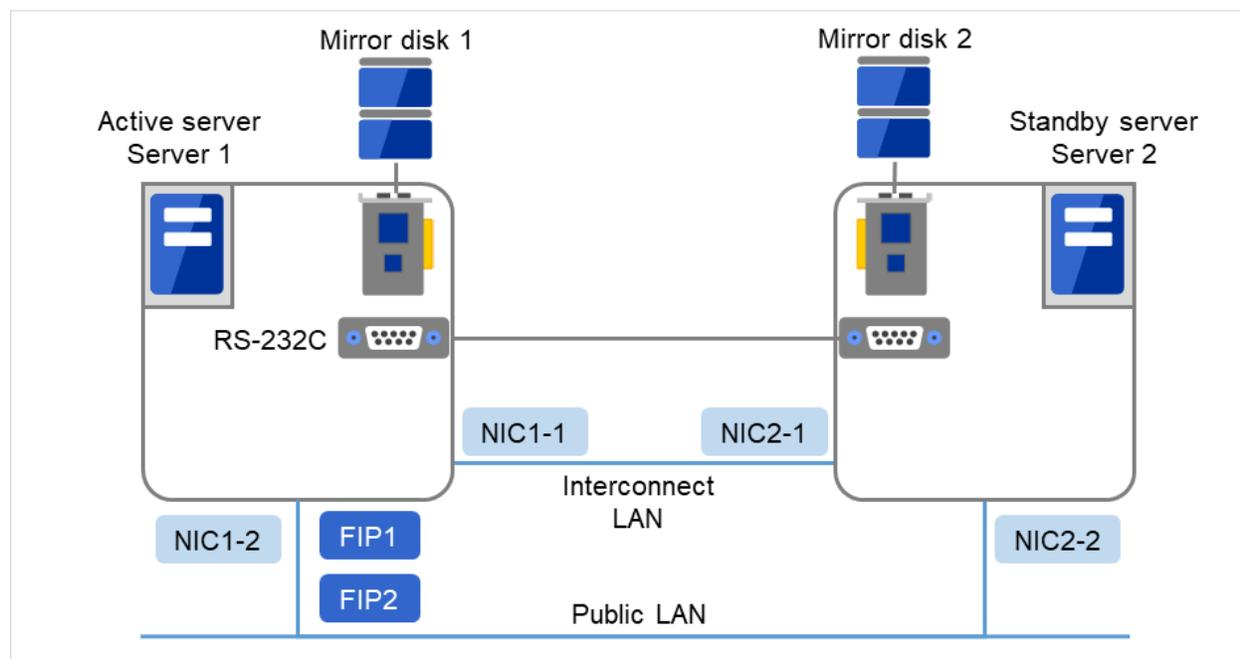
Fig. 3.9: Example of cluster configuration (2) (Mirror disk type)
