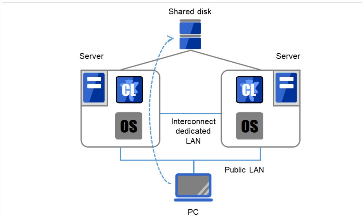
Fig. 2.6: System configuration
