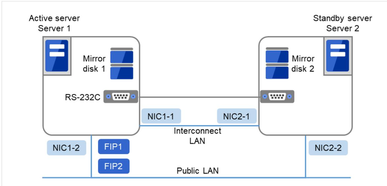
Fig. 3.8: Example of cluster configuration (1) (Mirror disk type)
