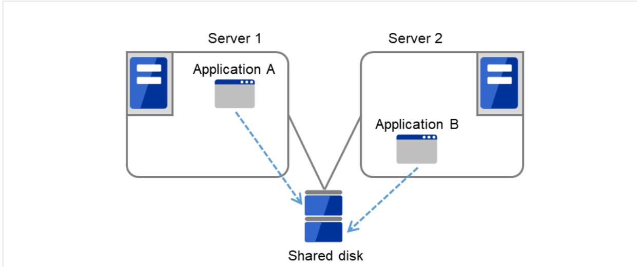
Fig. 2.11: Multi-directional standby cluster system with different applications (1)
