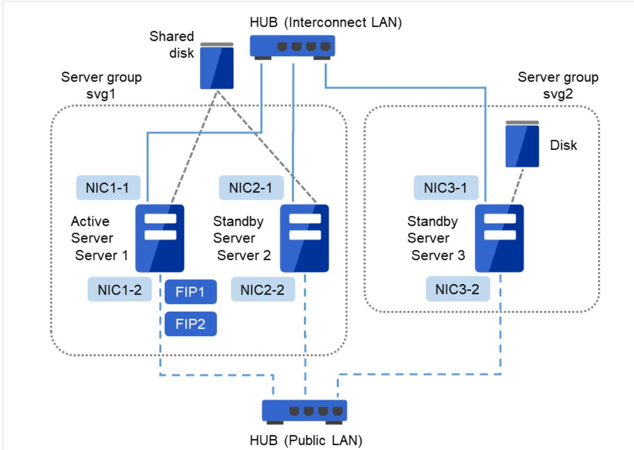
Fig. 3.10: Example of cluster configuration (Hybrid disk type)
