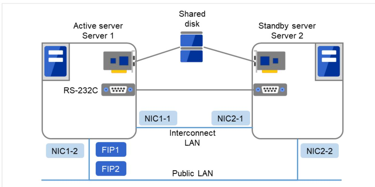
Fig. 3.7: Example of cluster configuration (Shared disk type)
