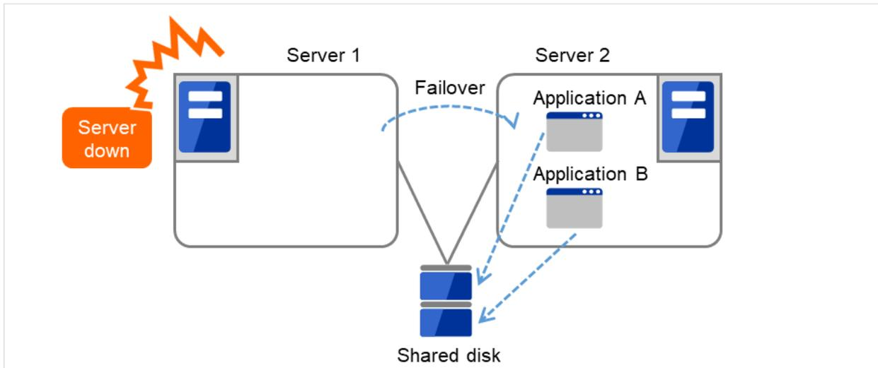
Fig. 2.12: Multi-directional standby cluster system with different applications (2)
