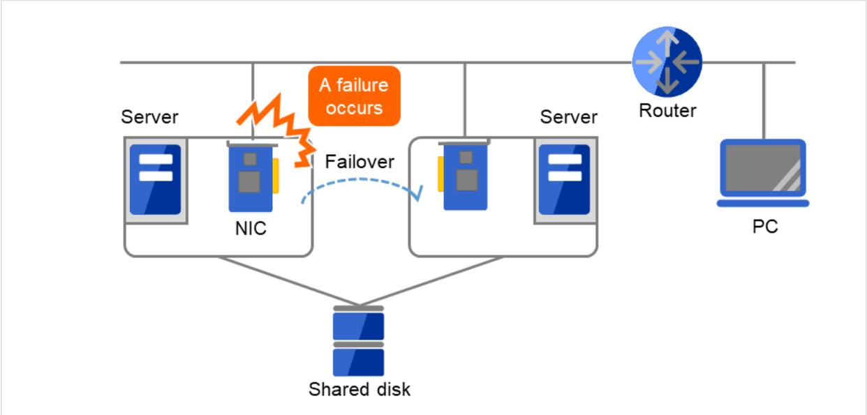
Fig. 2.21: Example of a failure with LAN (NIC)
