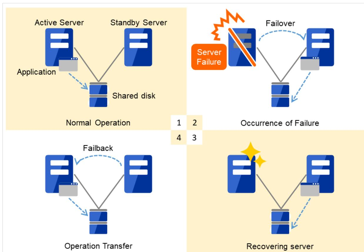
Fig. 2.2: From occurrence of a failure to recovery
